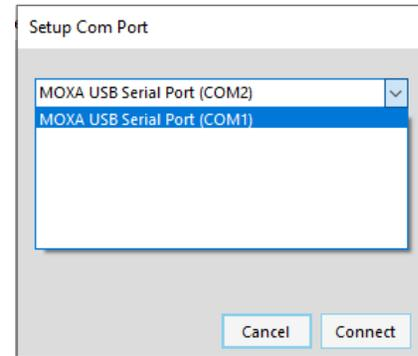
3. Selecting 'Connect' starts a search for a connected HM Configurator and displays the unit's configuration once it is detected.
