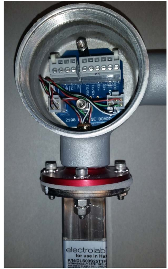
Figure 1. Model 2100 Digital Level Sensor (on left with blue flange) Model 2100 with High Level Shut-In (on right with red flange)
