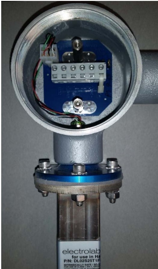
Figure 1. Model 2100 Digital Level Sensor (on left with blue flange) Model 2100 with High Level Shut-In (on right with red flange)
