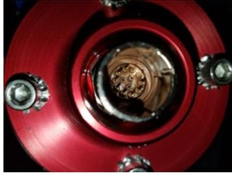
HLS sensor connector with 13 pins
