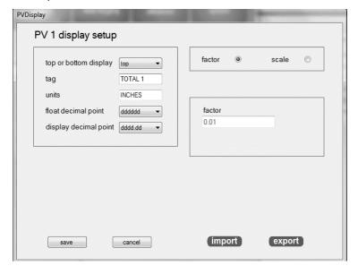
For 32 bit modbus, the TankChek LCD210 reads the raw Modbus RTU data and uses a factor of 1, (float). In this case, the data is simply formatted to the proper display with the use of the "display decimal point" selection of "dddd.dd".
