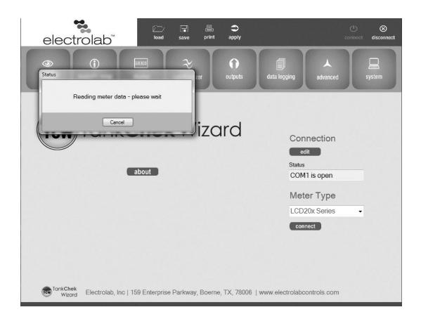
In the event more than one LCD Display is used on a RS485 communications line, each will need a unique scanner ID for the TankChek Wizard to communicate with it; this will need to be **configured manually via the push buttons**.
