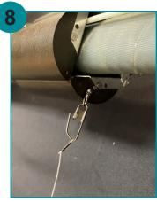
Connect the HLS test fixture wire to the high-level float and close the clip pin. Sensor is ready for communications test and installation!
