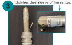
Slide the cord grip/HLS bushing assembly onto the sleeve 1-foot from the top of the sensor. Align the test fixture tube with the break in the sensor label and the ground screw.
