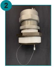
Apply thread sealant to the threads of the cord grip & the threads of the reducer bushing. Join the two components together.
