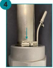
Slide the stainless steel hose clamp onto the sleeve of the sensor, right above the cord grip/reducer assembly. Tighten the screw on the opposite side
