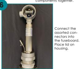
Tighten the housing onto the sensor flange. Feed the pigtail through the 1-inch port of the housing. Do **not** allow the wires to twist as the housing is screwed in place.
