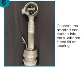
Tighten the housing onto the sensor flange. Feed the pigtail through the 1-inch port of the housing. Do not allow the wires to twist as the housing is screwed in place.
