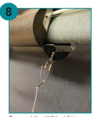
Connect the HLS test fixture wire to the high-level float and close the clip pin. Sensor is ready for communications test and installation!
