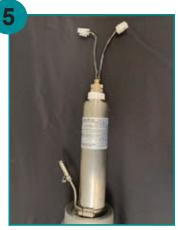
Apply thead sealant to the threads of the sensor flange. Remove the pigtail from the housing and connect the rounded end to the top of the sensor flange.
