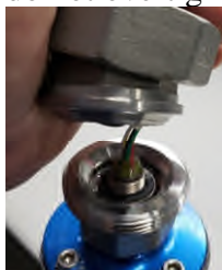
Ensure cable is not caught in threads or joint
