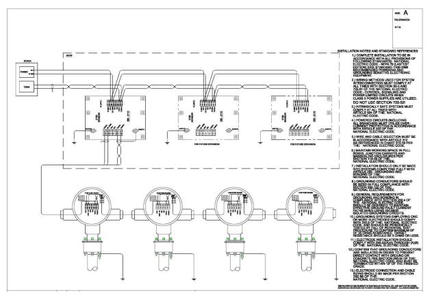
Figure 3. DLS2100 Connection Diagram
