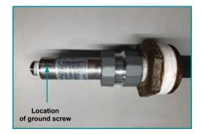
Remove the ground screw from the sleeve of the sensor. Slide the cord grip/reducer bushing assembly onto the sleeve 1-foot from the top of the sensor. Tighten the cord grip/reducer
