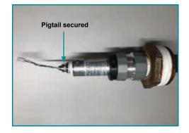
Apply thead sealant to the threaded area of the sensor flange. Remove pigtail from sensor housing and connect the rounded end to the top of the sensor flange.
