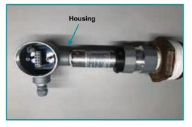
Feed pigtail through housing's 1-inch port. Tightenhousing into the sensor flange (do not allow the wires to twist). Connect the associated connectors into the fuseboard. Sensor is ready for communications test and installation.
