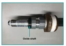
Slide the black, oxide shaft collar onto the stainless steel sleeve of the sensor, right above the cord grip/reducer assembly. Tighten the side bolts of the shaft collar to prevent slipping. Replace the ground screw.
