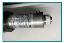
Hold the 2110EX over the top of the sensor. Screw circular connector onto the connector of the top plug.
