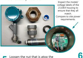
Apply thread sealant to the threads of the cord grip & reducer bushing. Join the two components together.
