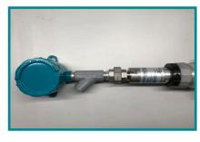
Join the 2110EX housing's 1" union with the top plug of the sensor, ensuring no wires are clipped in the process. Tighten to secure.
