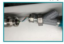
9 Remove lower section of the 1" union and secure it to the sensor threads.
